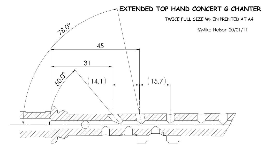
This drawing shows the dimensions for spreading the top 3 finger holes apart so as to make the playing of concert pitch chanters easier by the chubbier finger.
